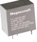
Electromechanical Relay | SPDT                  | 15 A           | 277 Vac<br>28 Vdc  | 100 mA                        | 25 ms         |
